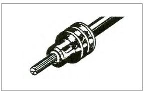
2. Align seal with cable insulation.
